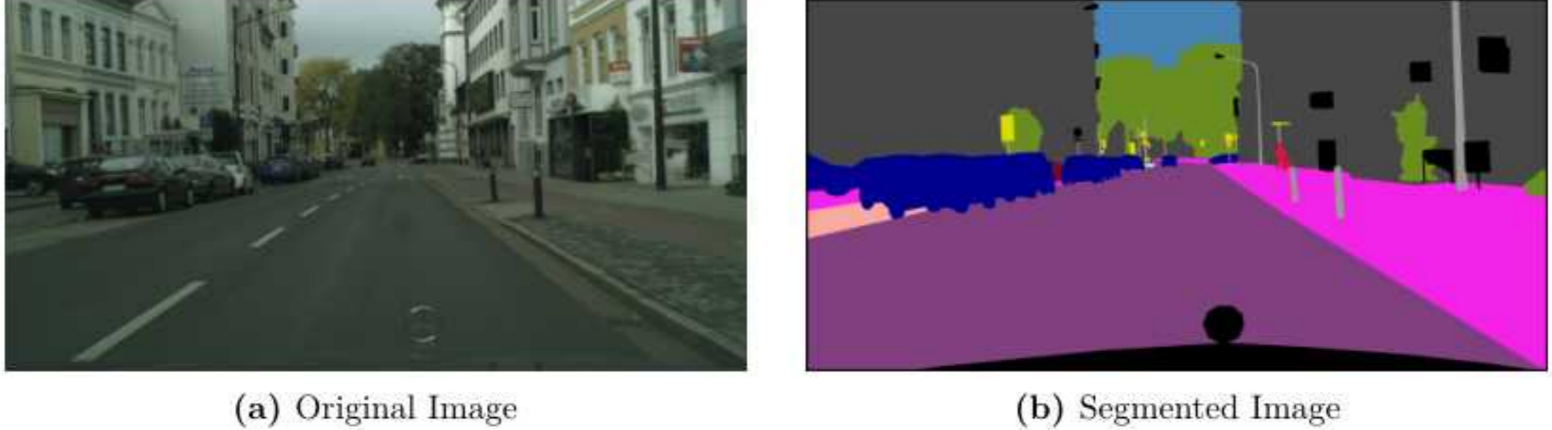
Figure 6 – Example of the segmentation process: traffic elements (purple, pink, yellow, and dark blue), sky (light blue), buildings (grey), and greenery (green)
